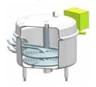
The large, continuously recharging stainless steel boiler, with its 1.5 I capacity and 3200 W heating element, can produce up to  $4.5 \, \text{kg H}_2\text{O/h}$  of steam.
