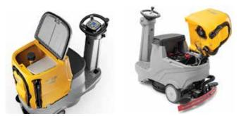
Maintenance is practical and simple, even for less experienced users. The recovery tank, vacuum filter and debris tray are easily accessible for immediate cleaning. The battery and charger compartment is also easily accessible for the user.
