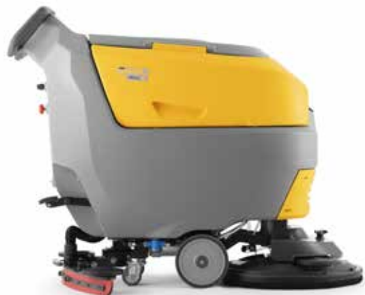
REXA 50 SD 55, the driven model, in a simplified version, with a 21" single brush
