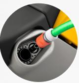
Water Stop: fast filling of the solution tank with automatic stop (optional).
