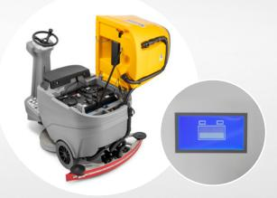
Even in this step, an immediate feedback of the state of battery charge is displayed on the screen.
