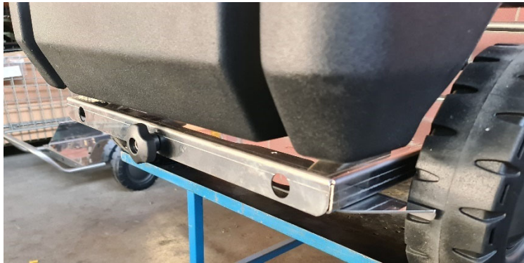
Detail of the brake knob being locked on the rear axle
